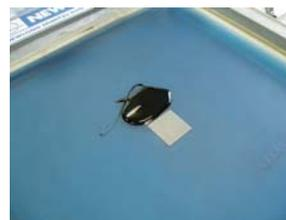
④ Filling catalyst paste in the pattern of the printing plate
