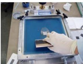
⑤ Filling catalyst paste in the pattern of the printing plate
