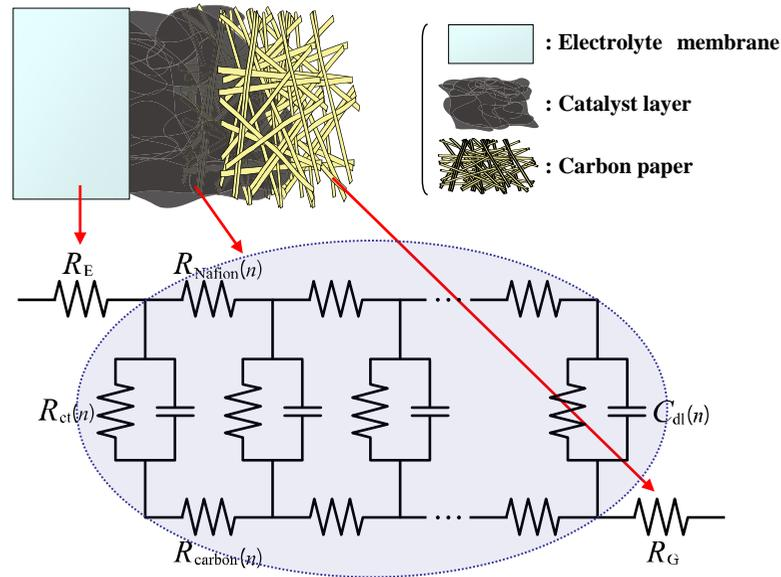
$R_{ct}(n)$  : Charge transfer resistance ( $\Omega$ )     $R_E$  : Electrolyte membrane resistance ( $\Omega$ )
