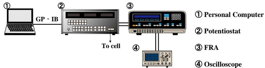
Fig. 7 Schematic diagram of the experimental apparatus
