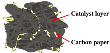
Fig. 1 Illustration of carbon paper coated by catalyst layer
