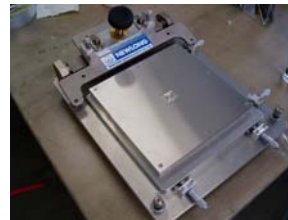
Fig. 2 Hand screen-printer designed for the fabrication of MEA (HP-320, NEWLONG Seimitsu Kogyo co., ltd.)
